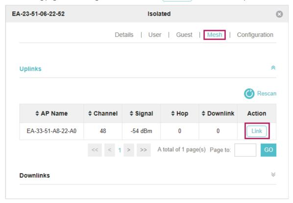
Once adoption has finished, your device can be managed by the controller in the same way as a wired EAP. You can click the EAP's name on the Access Points tab to view and configure the mesh parameters of the EAP on the pop-up window. Please refer to <u>View Mesh Information of the EAP</u>.
